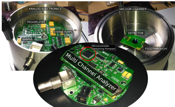
Figure: Vacuum chamber showing the detector housing assembly and electrical feedthrough. The MCA is stacked on the analog electronics.
