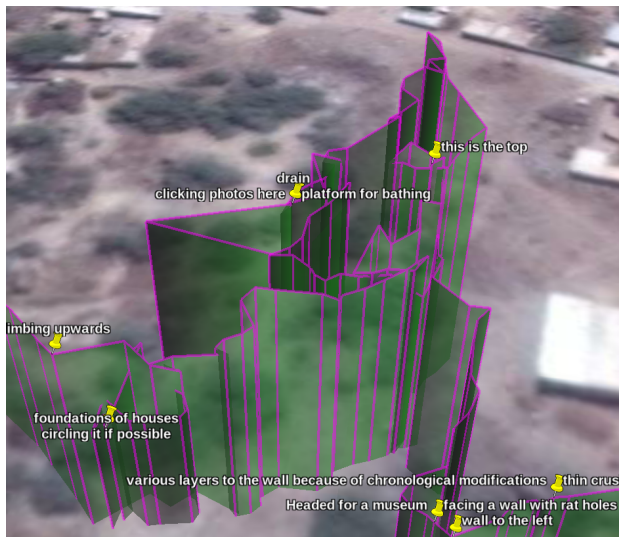
FIG. 6: An attempt to recreate the contours of a series of excavated houses shows the limitations of mobile GPS. An error margin of about 1 metre obfuscates the positions of the wall boundaries that I had attempted to trace. Elevation data suffers from similar precision errors, but the slope being gradual, the error margin is more acceptable. The measured coordinates being absolute, visualization of several such paths on a common platform will provide a clearer picture.
