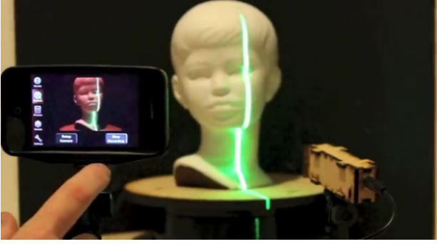
FIG. 9: 3D scanning using a smartphone and a line laser
